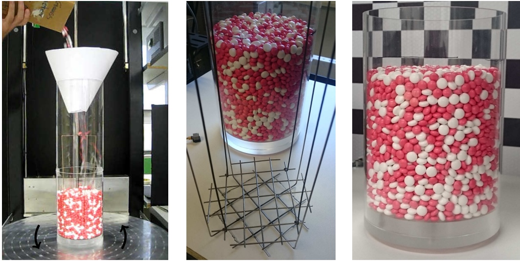
Figure 2.1: Loose packing preparation: (left) During the initial filling the container is rotated on a motorized platform. (middle) The two grids have been pulled out slowly to create a loose packing with random particle orientations. (right) Final loose packing.
